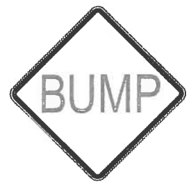
SIGN ADJACENT TO SPEED LUMP (IN BOTH DIRECTIONS)
