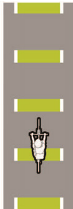
Figure 3.7. Intersection pavement markings are designed to improve visibility, alert all roadway users of expected behaviors, and reduce conflicts with turning vehicles.
